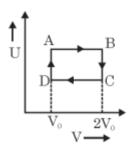
The temperature of the gas at B and C are 500 K and 300 K, respectively. The heat absorbed by the gas (in kcal) in this cyclic process is:
